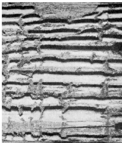
Figure 3-4. Termite-damaged wood. Figure 3-4. Carpenter ant-damaged wood.
