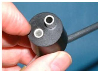
To use the device, just place the long tube beside a small insect, put the rubber tube into your mouth and suck sharply. With a bit of practice, you will find that this is an excellent way to collect smaller insects with ease.
