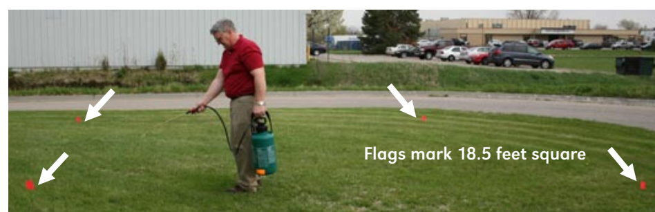
Measure a test area 18.5 feet x 18.5 feet square. Then spray in the manner you would normally do and record the time in seconds to "treat" the test area.
