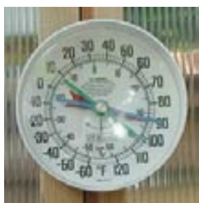
Minimum-Maximum thermometers show current temperature and the highest and lowest temperature since reset.
