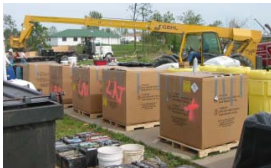
After sorting, hazardous waste was packed in large, extra strong boxes with double-wall construction for safe transport.
