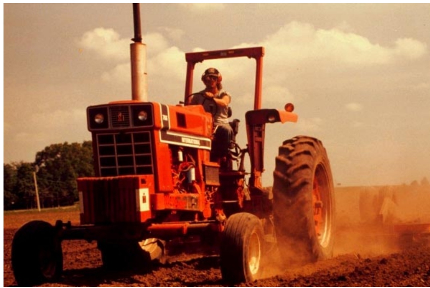
Roll-over protective structures (ROPS) for tractors come in a variety of styles including this simple two-post design.
